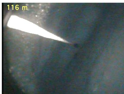
**Figure 2.** Photograph from borehole video camera showing typical open fracture. Fracture depth is 116 m below the ice surface. Vertical bright line is a signal cable which can be seen entering the borehole at the base of the fracture.
