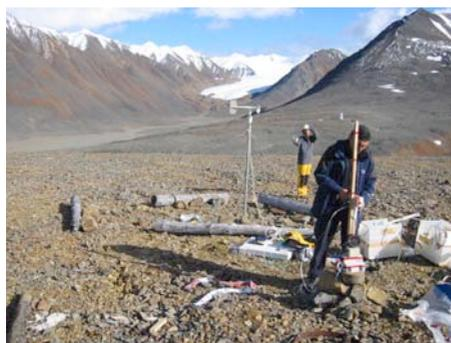
**Figure 3.** Meteorological station at No.31 Glacier. Thermometer, anemometer, solar radiation meter and snow-depth camera were installed.
