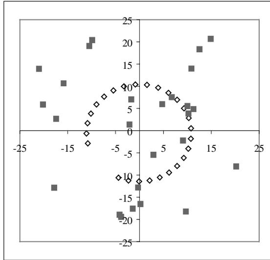
**Figure 1.** Astrometric signal of a 1 Uranus mass object in a 5 AU orbit about a 1 solar mass star at a distance of 20 pc. Diamonds represent the true values, while squares are 10 years' worth of measurements at 150 day intervals, with 25  $\mu\text{as}$  errors; both axes are in  $\mu\text{as}$ . Simple Monte Carlo modelling indicates such an object is easily detectable from the data.
